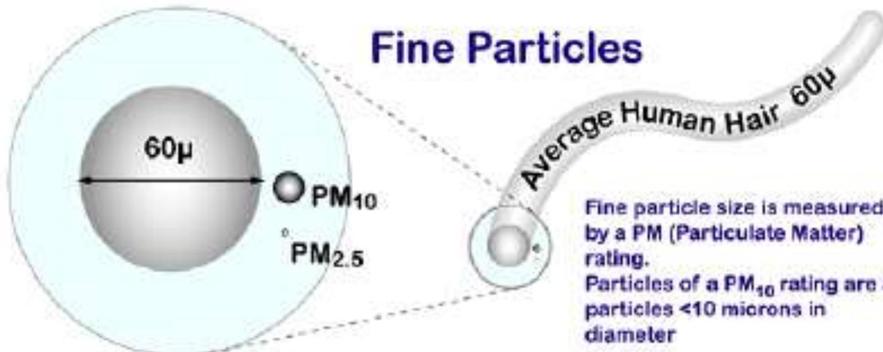
Fine particle size is measured by a PM (Particulate Matter) rating. Particles of a PM<sub>10</sub> rating are all particles <10 microns in diameter
